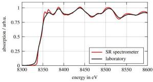
X-ray absorption spectrum of a 6um-thick Ni foil. Comparison to the spectrum obtained at a synchrotron (NSLS, resolving power  $E/\Delta E = 5000$ ) shows the high quality results of the tabletop instrument.
