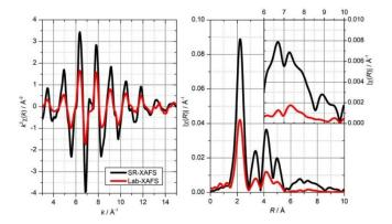
Sample XAFS measurement of a 10um Cu foil, comparing lab-based (red) and synchrotron (black) results. EXAFS oscillations (left) and corresponding Fourier transformation (right).
