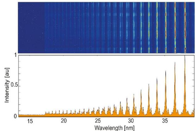
Sample measurement demonstrating the resolving power of maxLIGHT. The shown high harmonic spectrum is generated by the interaction of a single femtosecond laser pulse with a solid target and subsequent spectral filtering. The substructure inherent to the generation process is clearly resolved by the XUV spectrometer.
